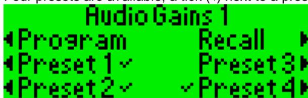
To **Recall** a virtual module preset, press and hold the **Recall** button, then press and release the desired **Preset** button. If the **Recall** button is released before the **Preset** button is released, nothing happens.
