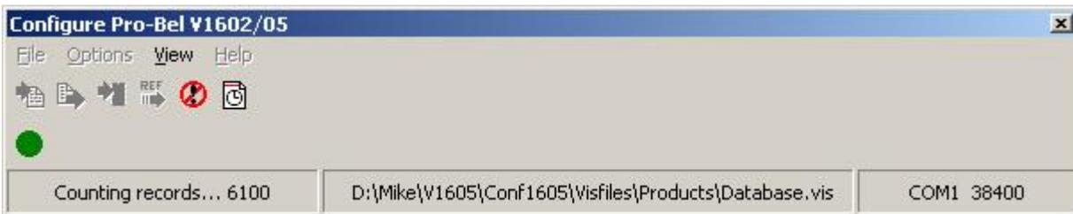
When the data transfer begins, the program uses the record count to initialise a progress bar so that the user is able to judge the progress of the data transfer.
