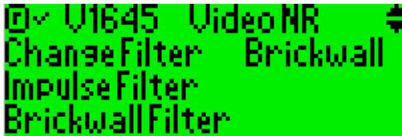
After selection of **Brickwall Filter**, the Brickwall Filter control screen is displayed:
